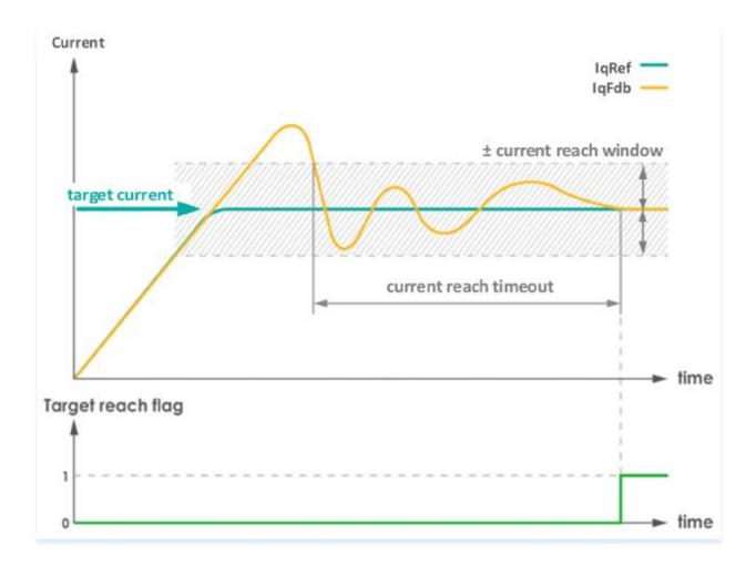
IqFdb refers to current feedback; likewise, velocity applies the same method to rise target reach flag and to determine whether the reference command is met. Please check <u>chapter 5.5.4 Target reach flag</u>
