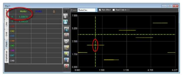
9. Keep moving curser and noting down all the Mark A x-axis values for the Theta table columns.
