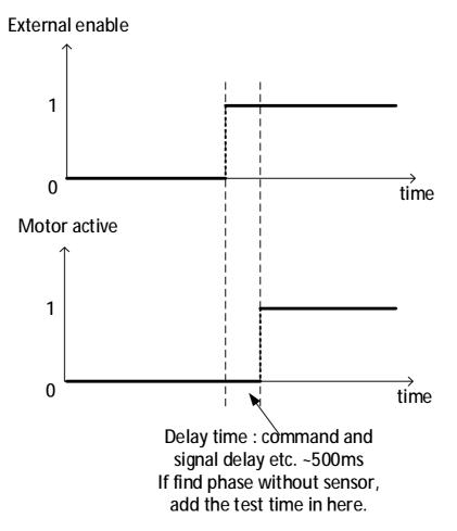
6. If users want to turn on the motor again after fault or quick stop occurs, only rising edge of external enable can do, see the diagram below.
