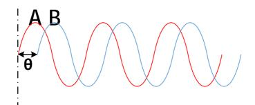
The sine and cosine signals can be drawn into a circle based on X (sine) and Y (cosine) co-ordinates and can therefore perform arctangent function (or, interpolation) to know the degree of theta in order to obtain finer position resolution.
