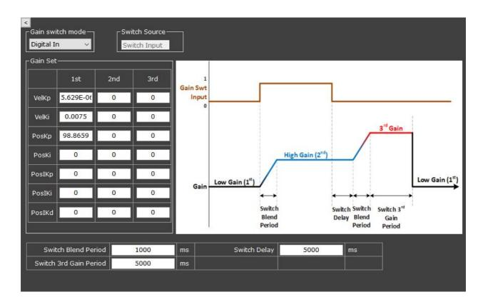
Use digital signal input to determine which gain-set to be applied.
