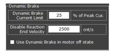
Brake motor by means of a controlled motor short circuit. This function can be applied both during motor-on and motor-off states, and can be used to:
