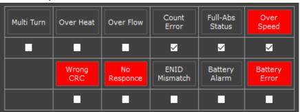
4 status flags have risen (represented in red) indicating the occurrence of encoder errors; yet, only the <u>selected</u> (shown as ticked) status flag "Over Speed" will be counted to trigger fault event.
