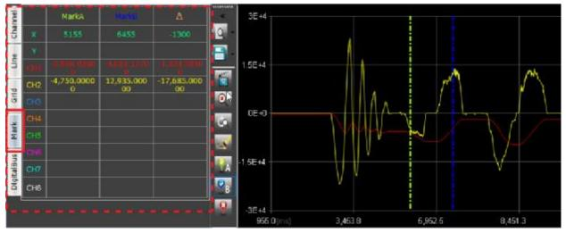
Mark tab shows the values and differences ( $\Delta$ ) of the marks A and B.
