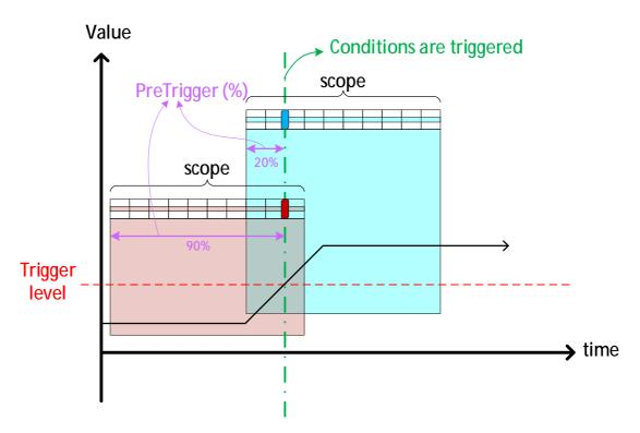
The scope on the left is with PreTrigger 90%, meaning that 90% of the data shown on the *left* scope is below trigger condition(s). Likewise, for the scope on the right, 20% of the data shown on the *right* scope is below trigger condition(s)
