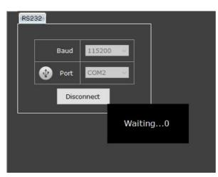
3. When the columns turn grey, it means the driver and the host computer are successfully connected.
