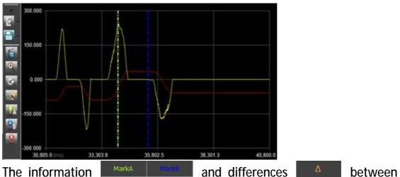
marks A and B are shown on the "Mark Tab" of Further Setting Panel.
